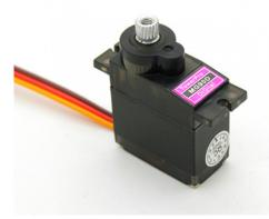
A small lightweight servo that is an upgraded version of the stalwart Towerpro MG90S digital servo but with more torque and greater speed. This little servo is perfect for aircraft, helicopters, mult-rotors, robots and other applications were you want a small, strong, fast servo. It is fitted with upgraded 6061-T6 aluminum gears and shafts and has a ballraced output.
